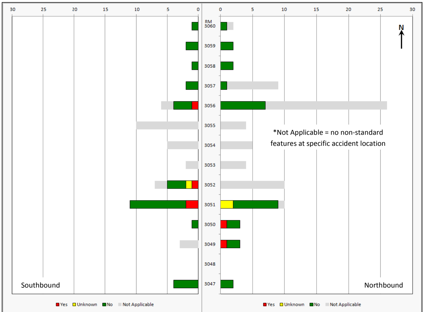
Figure 4 – Correlation of Total Number of Accidents for 3-Year Period to Non-Standard Features by I-81 Reference Marker
